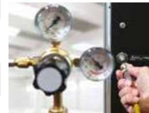
Nitrogen pressure control
